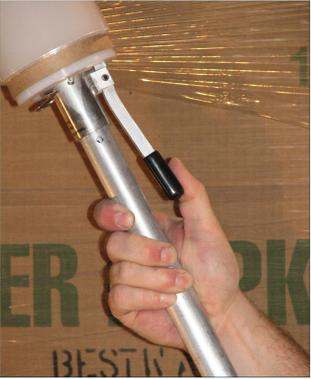
Tension controlled plus handbrake for the tightest possible wrap
