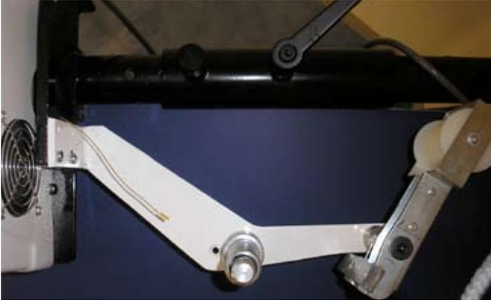
1b) Side view of Brake Arm connected to back of XL-2 machine
