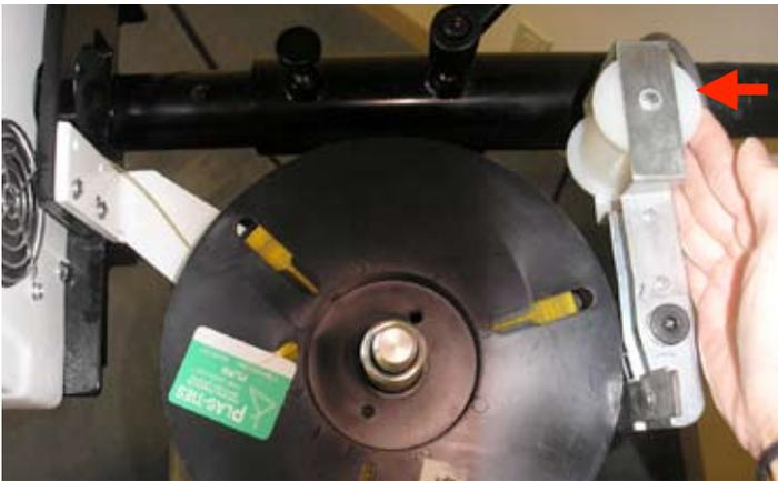
3) Pull end of tie out and under White Roller. Make sure that paper side of the tie is on the bottom and plastic side is on top.
