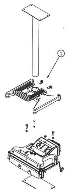
1. Insert standing tube into pedal base and fixed the short screw.
