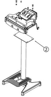
2. Use four long screws, connect enclosure body to standing tube.
