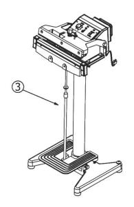
3. Attach puller tension rod to puller localized under lower sealing body and then attach to food pedal.
