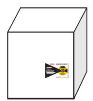
If the package is twice as long as it is wide, use two impact indicators. Place a second indicator in the same position on the opposite side of the package.
